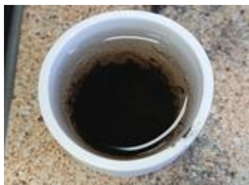
Fig. 2 Specimen in additional distilled water to solve KOH solvent.
