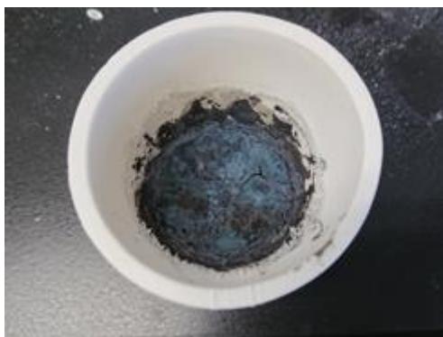
Fig. 1 Specimen after the first heat treatment with KOH.
